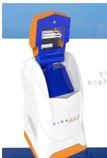
LytBot is a robot that uses pulsed Broad-Wavelength with Ultraviolet C (UVC) Light which can eliminate pathogens in seconds. The robot runs ultra-fast cycles, quickly and reliably targeting surface based pathogen load reducing the risk of infection spread. A single resident room, including the bathroom, can be disinfected in 15 minutes.
